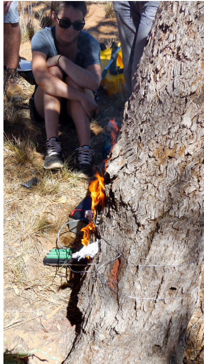
Experimental burn on Eucalyptus coolabah. Note flaming wick, thermocouples, data logger and stunned expression on the faces of the student pyromaniacs.
