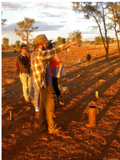
Extracting water from “No Name Bore” near Mudgeacca Station. In April 2010 the water table here was at about 21m below ground level. According to Philip Prince, owner of Mudgeacca, the bore was drilled to about 23m and was abandoned due to the saltiness of the water. It terminated in limestone.
