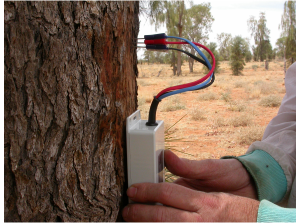
Installing a sap flow meter on the trunk of a waddi tree on Mudgeacca Station near Boulia.
