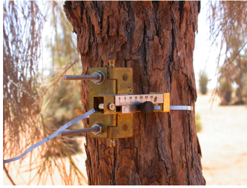
Band dendrometer measuring girth increment of waddi tree on Montague Downs Station
